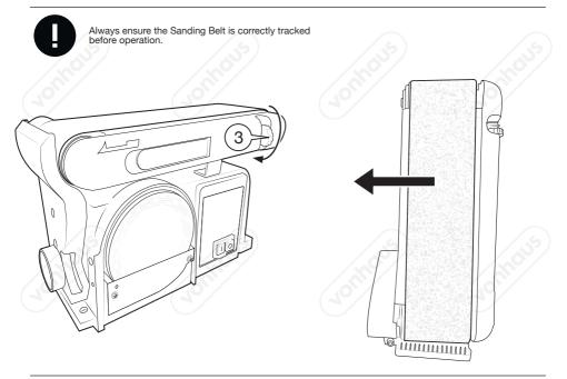
Ensure the sanding belt runs central to the rollers.
